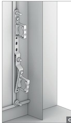
A - Align the bracket and mount it with washers and nuts to the sliding studs inserted in the 2 guides of the metal box
