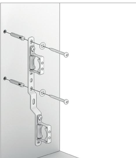
Drill the surface of the wall in correspondence with the slots on the metal bracket and fix with screws and expansion plugs \*
