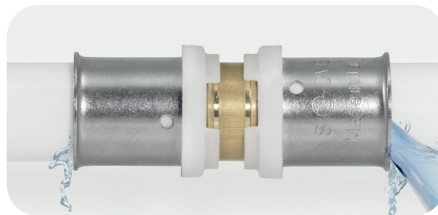
Fitting NOT pressed and tested between 1 and 4.5 bar* · IT LEAKS
